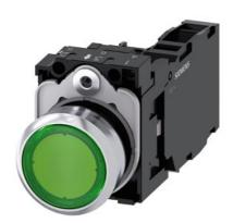
Illuminated pushbutton, 22 mm, round, metal, shiny, green, pushbutton, flat, momentary contact type, with holder, 1 NO+1 NC, LED module with integrated LED 110 V AC, screw terminal, with laser labeling, upper case and lower case, always upper case at beginning of line
