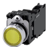
Illuminated pushbutton, 22 mm, round, metal, shiny, yellow, pushbutton, flat, momentary contact type, with holder, 1 NO+1 NC, LED module with integrated LED 110 V AC, spring-type terminal, with laser labeling, inscription or symbol Customer-specific selection with SIRIUS ACT configurator (CIN)
