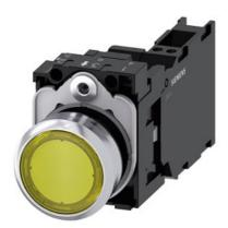
Illuminated pushbutton, 22 mm, round, metal, shiny, yellow, pushbutton, flat, momentary contact type, with holder, 1 NO+1 NC, LED module with integrated LED 110 V AC, spring-type terminal, with laser labeling, lower case
