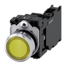
Illuminated pushbutton, 22 mm, round, metal, shiny, yellow, pushbutton, flat, momentary contact type, with holder, 1 NO+1 NC, LED module with integrated LED 110 V AC, spring-type terminal, with laser labeling, upper case
