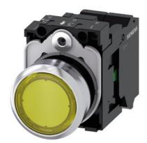
Illuminated pushbutton, 22 mm, round, metal, shiny, yellow, pushbutton, flat, momentary contact type, with holder, 1 NO, LED module with integrated LED 110 V AC, Spring-type terminal
