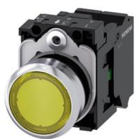
Illuminated pushbutton, 22 mm, round, metal, shiny, yellow, pushbutton, flat, momentary contact type, with holder, 1NO, LED module with integrated LED 110 V AC, spring-type terminal, with laser labeling, upper case and lower case, Always upper case at the beginning of the word
