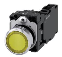
Illuminated pushbutton, 22 mm, round, metal, shiny, yellow, pushbutton, flat, momentary contact type, with holder, 1 NO+1 NC, LED module with integrated LED 110 V AC, screw terminal, with laser labeling, lower case
