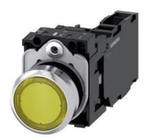
Illuminated pushbutton, 22 mm, round, metal, shiny, yellow, pushbutton, flat, momentary contact type, with holder, 1 NO+1 NC, LED module with integrated LED 110 V AC, screw terminal, with laser labeling, upper case and lower case, always upper case at beginning of line
