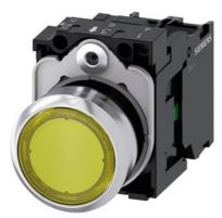
Illuminated pushbutton, 22 mm, round, metal, shiny, yellow, pushbutton, flat, momentary contact type, with holder, 1NO, LED module with integrated LED 110 V AC, screw terminal, with laser labeling, lower case
