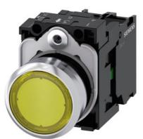
Illuminated pushbutton, 22 mm, round, metal, shiny, yellow, pushbutton, flat, momentary contact type, with holder, 1NO, LED module with integrated LED 110 V AC, screw terminal, with laser labeling, upper case and lower case, always upper case at beginning of line
