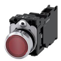
Illuminated pushbutton, 22 mm, round, metal, shiny, red, pushbutton, flat, momentary contact type, with holder, 1 NO+1 NC, LED module with integrated LED 110 V AC, spring-type terminal, Z=20-unit packaging
