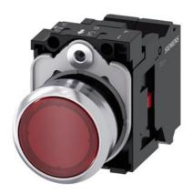
Illuminated pushbutton, 22 mm, round, metal, shiny, red, pushbutton, flat, momentary contact type, with holder, 1NC, LED module with integrated LED 110 V AC, spring-type terminal, with laser labeling, inscription or symbol Customer-specific selection with SIRIUS ACT configurator (CIN)
