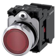
Illuminated pushbutton, 22 mm, round, metal, shiny, red, pushbutton, flat, momentary contact type, with holder, 1NC, LED module with integrated LED 110 V AC, spring-type terminal, with laser labeling, symbol number according to, ISO 7000 or IEC 60417
