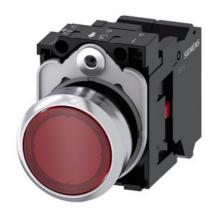
Illuminated pushbutton, 22 mm, round, metal, shiny, red, pushbutton, flat, momentary contact type, with holder, 1NC, LED module with integrated LED 110 V AC, spring-type terminal, with laser labeling, upper case
