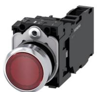
Illuminated pushbutton, 22 mm, round, metal, shiny, red, pushbutton, flat, momentary contact type, with holder, 1 NO+1 NC, LED module with integrated LED 110 V AC, screw terminal
