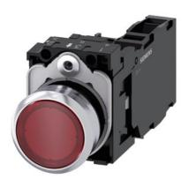
Illuminated pushbutton, 22 mm, round, metal, shiny, red, pushbutton, flat, momentary contact type, with holder, 1 NO+1 NC, LED module with integrated LED 110 V AC, screw terminal, with laser labeling, upper case and lower case, always upper case at beginning of line
