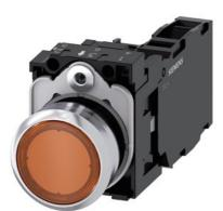
Illuminated pushbutton, 22 mm, round, metal, shiny, amber, pushbutton, flat, momentary contact type, with holder, 1 NO+1 NC, LED module with integrated LED 110 V AC, screw terminal, with laser labeling, lower case
