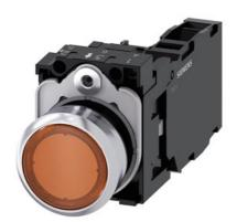
Illuminated pushbutton, 22 mm, round, metal, shiny, amber, pushbutton, flat, momentary contact type, with holder, 1 NO+1 NC, LED module with integrated LED 110 V AC, screw terminal, with laser labeling, upper case
