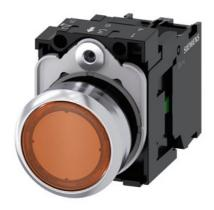
Illuminated pushbutton, 22 mm, round, metal, shiny, amber, pushbutton, flat, momentary contact type, with holder, 1 NO, LED module with integrated LED 110 V AC. screw terminal
