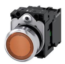
Illuminated pushbutton, 22 mm, round, metal, shiny, amber, pushbutton, flat, momentary contact type, with holder, 1NO, LED module with integrated LED 110 V AC, screw terminal, with laser labeling, symbol number according to, ISO 7000 or IFC 60417
