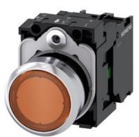
Illuminated pushbutton, 22 mm, round, metal, shiny, amber, pushbutton, flat, momentary contact type, with holder, 1NO, LED module with integrated LED 110 V AC, screw terminal, with laser labeling, lower case
