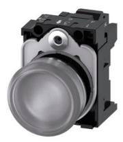
Indicator lights, 22 mm, round, metal, shiny, clear, lens, smooth, with holder, LED module with integrated LED 24 V AC/DC, spring-type terminal, with laser labeling, upper case and lower case, always upper case at the beginning of the word
