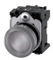
Indicator lights, 22 mm, round, metal, shiny, clear, lens, smooth, with holder, LED module with integrated LED 24 V AC/DC, screw terminal, with laser labeling, lower case
