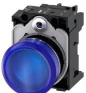
Indicator lights, 22 mm, round, metal, shiny, blue, lens, smooth, with holder, LED module with integrated LED 24 V AC/DC, screw terminal, with laser labeling, inscription or symbol Customer-specific selection with SIRIUS ACT configurator (CIN)
