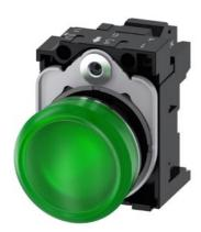
Indicator lights, 22 mm, round, metal, shiny, green, lens, smooth, with holder, LED module with integrated LED 24 V AC/DC, spring-type terminal, with laser labeling, upper case and lower case, always upper case at the beginning of the word
