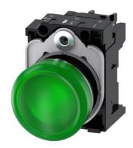
Indicator lights, 22 mm, round, metal, shiny, green, lens, smooth, with holder, LED module with integrated LED 24 V AC/DC, screw terminal, with laser labeling, lower case
