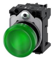
Indicator light, 22 mm, round, metal, shiny, green, lens, smooth, with holder, LED module with integrated LED 24 V AC/DC, screw terminal, with laser labeling, upper case and lower case, always upper case at beginning of line
