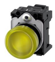
Indicator lights, 22 mm, round, metal, shiny, yellow, lens, smooth, with holder, LED module with integrated LED 24 V AC/DC, spring-type terminal, with laser labeling, upper case
