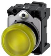
Indicator lights, 22 mm, round, metal, shiny, yellow, lens, smooth, with holder, LED module with integrated LED 24 V AC/DC, spring-type terminal, Z=20-unit packaging
