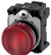
Indicator lights, 22 mm, round, metal, shiny, red, lens, smooth, with holder, LED module with integrated LED 24 V AC/DC, spring-type terminal, with laser labeling, inscription or symbol Customer-specific selection with SIRIUS ACT configurator (CIN)
