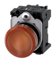
Indicator lights, 22 mm, round, metal, shiny, amber, lens, smooth, with holder, LED module with integrated LED 24 V AC/DC, screw terminal, with laser labeling, upper case
