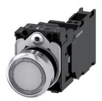
Illuminated pushbutton, 22 mm, round, metal, shiny, clear, pushbutton, flat, momentary contact type, with holder, 1 NO+1 NC, LED module with integrated LED 24 V AC/DC, spring-type terminal, with laser labeling, symbol number according to, ISO 7000 or IEC 60417
