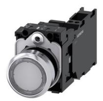
Illuminated pushbutton, 22 mm, round, metal, shiny, clear, pushbutton, flat, momentary contact type, with holder, 1 NO+1 NC, LED module with integrated LED 24 V AC/DC, spring-type terminal, with laser labeling, lower case
