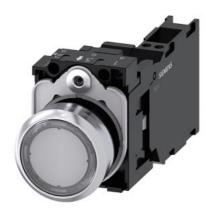
Illuminated pushbutton, 22 mm, round, metal, shiny, clear, pushbutton, flat, momentary contact type, with holder, 1 NO+1 NC, LED module with integrated LED 24 V AC/DC, spring-type terminal, Z=20-unit packaging
