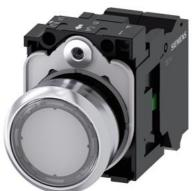
Illuminated pushbutton, 22 mm, round, metal, shiny, clear, pushbutton, flat, momentary contact type, with holder, 1NO, LED module with integrated LED 24 V AC/DC, spring-type terminal, with laser labeling, inscription or symbol Customer-specific selection with SIRIUS ACT configurator (CIN)
