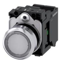
Illuminated pushbutton, 22 mm, round, metal, shiny, clear, pushbutton, flat, momentary contact type, with holder, 1NO, LED module with integrated LED 24 V AC/DC, spring-type terminal, with laser labeling, lower case
