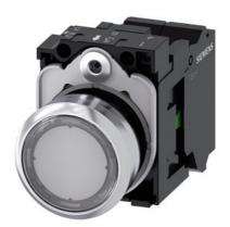
Illuminated pushbutton, 22 mm, round, metal, shiny, clear, pushbutton, flat, momentary contact type, with holder, 1NO, LED module with integrated LED 24 V AC/DC, spring-type terminal, with laser labeling, upper case
