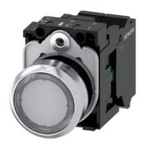
Illuminated pushbutton, 22 mm, round, metal, shiny, clear, pushbutton, flat, momentary contact type, with holder, 1NO, LED module with integrated LED 24 V AC/DC, spring-type terminal, with laser labeling, upper case and lower case, always upper case at beginning of line
