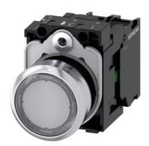
Illuminated pushbutton, 22 mm, round, metal, shiny, clear, pushbutton, flat, momentary contact type, with holder, 1NO, LED module with integrated LED 24 V AC/DC, screw terminal, with laser labeling, symbol number according to, ISO 7000 or IFC 60417
