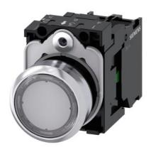
Illuminated pushbutton, 22 mm, round, metal, shiny, clear, pushbutton, flat, momentary contact type, with holder, 1NO, LED module with integrated LED 24 V AC/DC, screw terminal, Z=20-unit packaging
