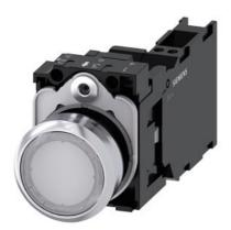
Illuminated pushbutton, 22 mm, round, metal, shiny, white, pushbutton, flat, momentary contact type, with holder, 1 NO+1 NC, LED module with integrated LED 24 V AC/DC, spring-type terminal, with laser labeling, inscription or symbol Customer-specific selection with SIRIUS ACT configurator (CIN)
