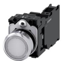
Illuminated pushbutton, 22 mm, round, metal, shiny, white, pushbutton, flat, momentary contact type, with holder, 1 NO+1 NC, LED module with integrated LED 24 V AC/DC, spring-type terminal, with laser labeling, upper case and lower case, Always upper case at the beginning of the word
