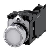
Illuminated pushbutton, 22 mm, round, metal, shiny, white, pushbutton, flat, momentary contact type, with holder, 1 NO+1 NC, LED module with integrated LED 24 V AC/DC, spring-type terminal, with laser labeling, symbol number according to, ISO 7000 or IEC 60417
