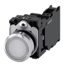
Illuminated pushbutton, 22 mm, round, metal, shiny, white, pushbutton, flat, momentary contact type, with holder, 1 NO+1 NC, LED module with integrated LED 24 V AC/DC, spring-type terminal, with laser labeling, upper case and lower case, always upper case at beginning of line
