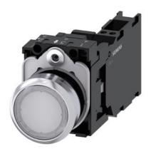
Illuminated pushbutton, 22 mm, round, metal, shiny, white, pushbutton, flat, momentary contact type, with holder, 1 NO+1 NC, LED module with integrated LED 24 V AC/DC, spring-type terminal, Z=20-unit packaging
