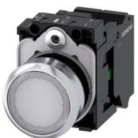
Illuminated pushbutton, 22 mm, round, metal, shiny, white, pushbutton, flat, momentary contact type, with holder, 1NO, LED module with integrated LED 24 V AC/DC, spring-type terminal, with laser labeling, inscription or symbol Customer-specific selection with SIRIUS ACT configurator (CIN)
