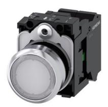
Illuminated pushbutton, 22 mm, round, metal, shiny, white, pushbutton, flat, momentary contact type, with holder, 1NO, LED module with integrated LED 24 V AC/DC, spring-type terminal, with laser labeling, symbol number according to, ISO 7000 or IEC 60417
