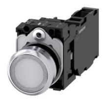
Illuminated pushbutton, 22 mm, round, metal, shiny, white, pushbutton, flat, momentary contact type, with holder, 1 NO+1 NC, LED module with integrated LED 24 V AC/DC, screw terminal, with laser labeling, upper case and lower case, Always upper case at the beginning of the word
