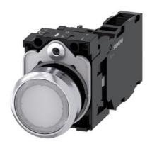
Illuminated pushbutton, 22 mm, round, metal, shiny, white, pushbutton, flat, momentary contact type, with holder, 1 NO+1 NC, LED module with integrated LED 24 V AC/DC, screw terminal, with laser labeling, symbol number according to, ISO 7000 or IEC 60417
