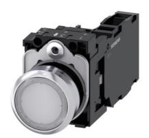
Illuminated pushbutton, 22 mm, round, metal, shiny, white, pushbutton, flat, momentary contact type, with holder, 1 NO+1 NC, LED module with integrated LED 24 V AC/DC, screw terminal, with laser labeling, upper case
